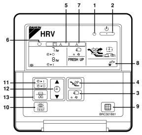
BRC301B61: Remote controller for VRV
