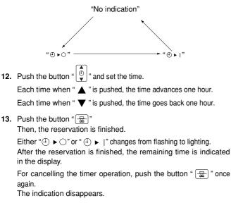
Operating the HRV unit using the remote controller of the VRV-system air conditioner
